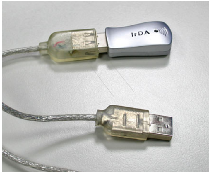
Step 2 – Locate the infrared sensor, and plug it into your Computer's USB port
